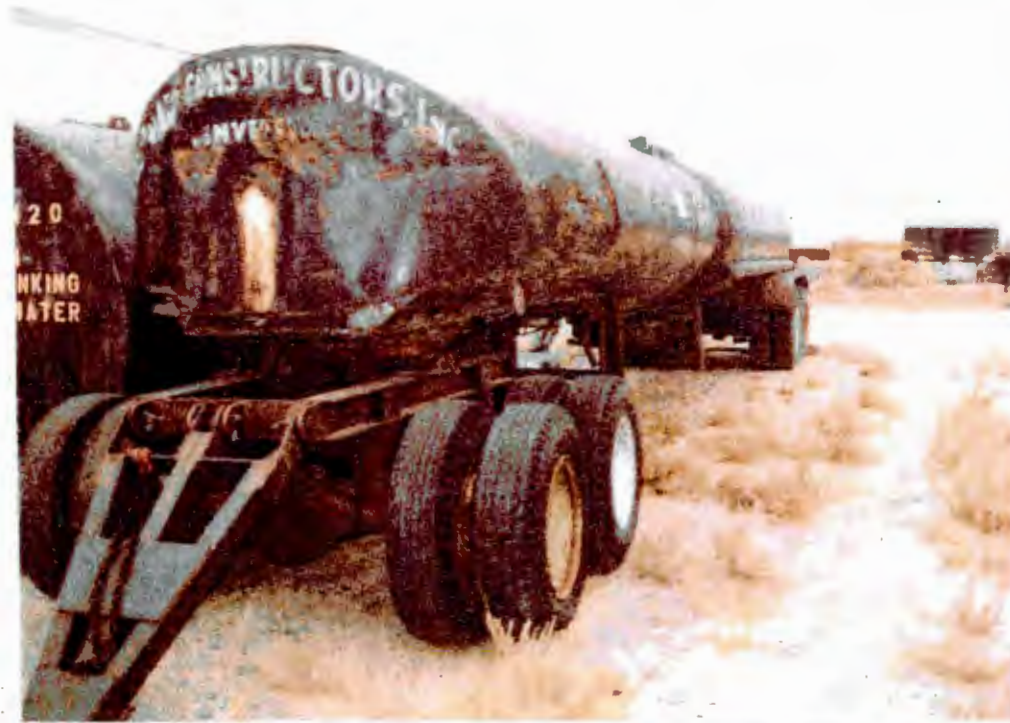
Photograph 2: View of Unit 70.118 5,450-gallon tack oil trailer.
