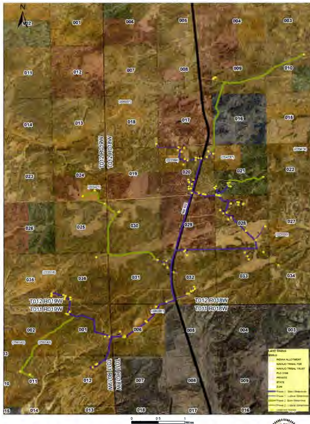
Exhibit V-4 Chichiltah-Vanderwagon Water Project Conceptual Layout
