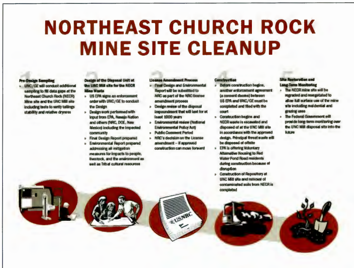
Figure 4. Cleanup Processes for the Northeast Church Rock Mine Site
