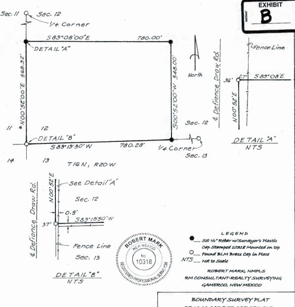
CERTIFICATE: I hereby certify that this Survey Plat shown hereon is prepared from an actual field survey performed by me; that the survey meets the Minimum Standard for land Surveys in New Mexico and that the survey is true and Correct to the best of my knowledge and belief.
