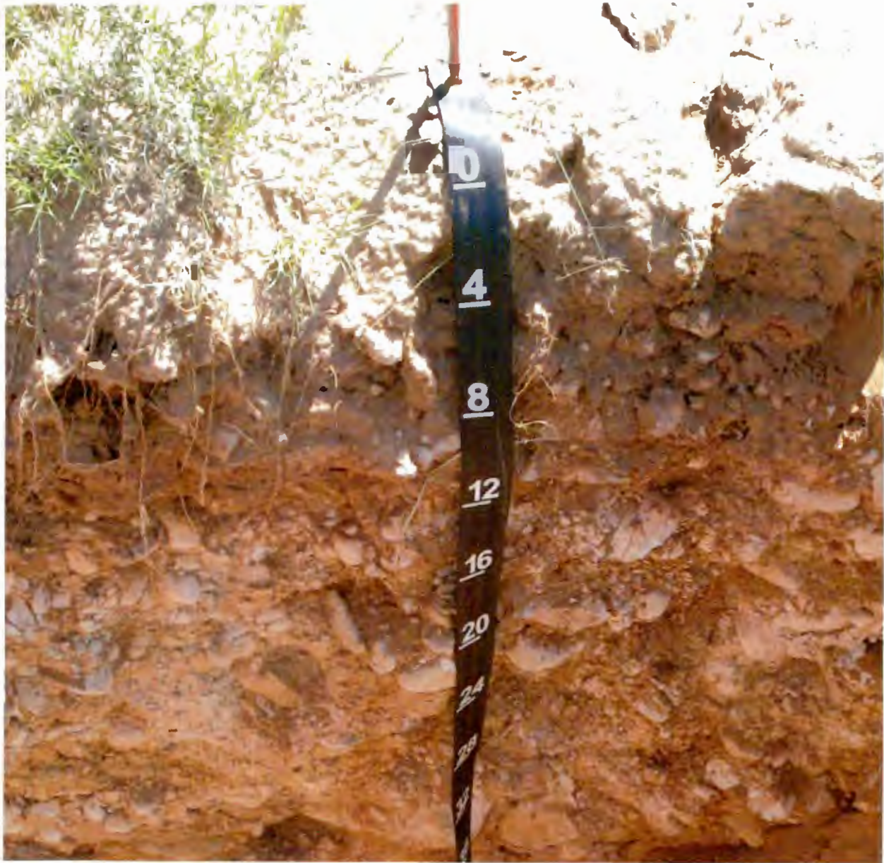
Photo 1. Pit 14- Topsoil to 10 inches, Gravel/Cobble to 50+ inches Photo 2.
